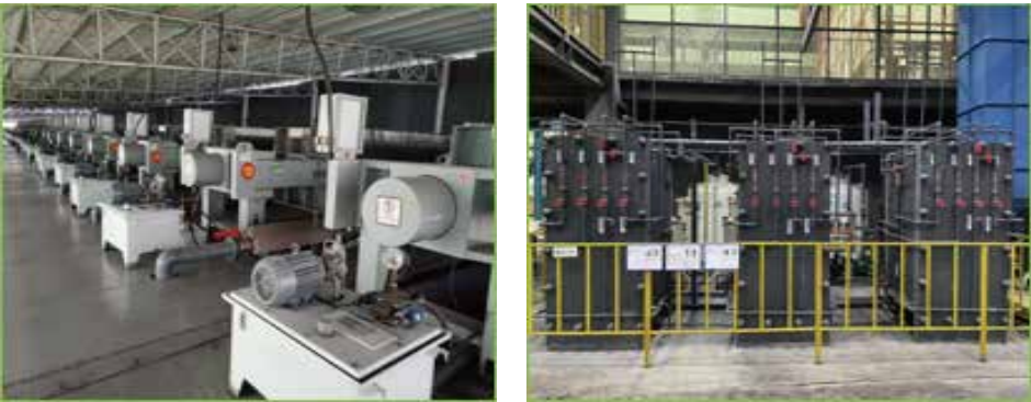
Above: Compression filtration replacing physiochemical system and diffusion dialysis acid recovery system
